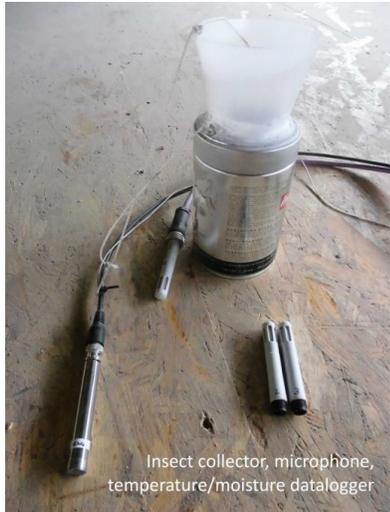
Insect collector, microphone, temperature/moisture datalogger
